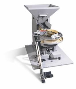
The Riley Automation range of product handling equipment includes vibratory, rotary and elevating parts feeders which take product from bulk storage through the processes of singulation, orientation and transportation to the next stage.
